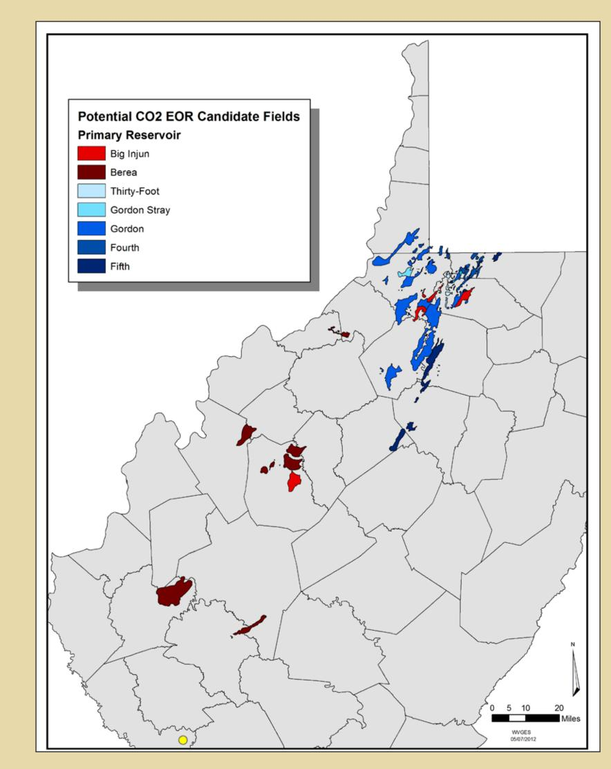
Depleted oil fields in West Virginia with reservoir depth greater than 2500ft (miscible flood) and/or reservoir pressure exceeding 1000psi. These fields would be targets for tertiary recovery via miscible CO₂ floods.
