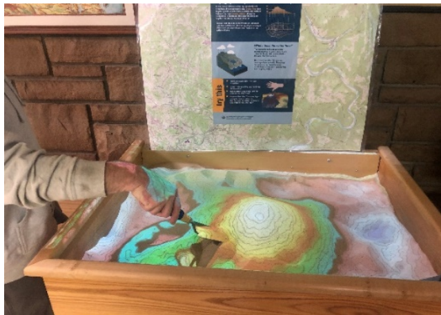
The Augmented Reality Sandbox: A computer projector overlays an interactive topographic map onto sand. By modifying the sand, visitors learn how geomorphologic processes change a landscape and how that landscape is represented on a topographic map
